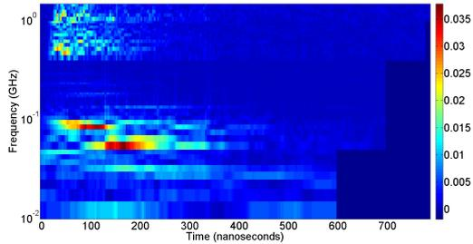
Figure 8: Time-dependant Nyquist limited Fourier transform analysis of the experimental EMP data of figure 2. The padding of the shorter arrays can be seen on the right of the figure, and more prominently in the lower frequencies. The 5% magnitude value was chosen in order to highlight that this region is not analysed data, whilst not disrupting the colourbar scales.
