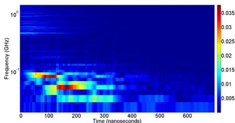
Figure 3: Time-dependant Fourier transform analysis of the EMP trace of figure 2, at bin length of 100 ns; optimal for low frequencies on the order of 10 MHz. The bin length is too long to adequately represent the high frequencies, and therefore any useful time information within this band is nullified.
