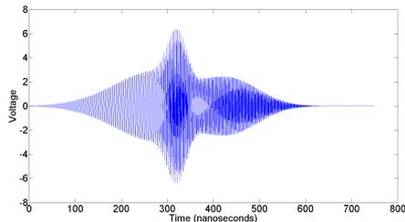
Figure 5: Test data created using a combination of sinusoidal waves and Gaussian peaks to produce a pre-determined waveform in intensity, frequency and time.
