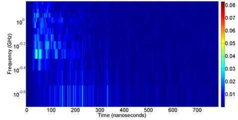
Figure 4: Time-dependant Fourier transform analysis of the EMP trace of figure 2, at bin length of 10 ns. The difference in  $y$  axis scaling with respect to figure 3 is due to the smaller bin size being unable to resolve frequencies on the same order of magnitude. This also accounts for the lack of the low frequency bursts seen in figure 3, as the EMP of lower frequencies has not undergone the necessary 2 period oscillation dictated by the Nyquist theorem.
