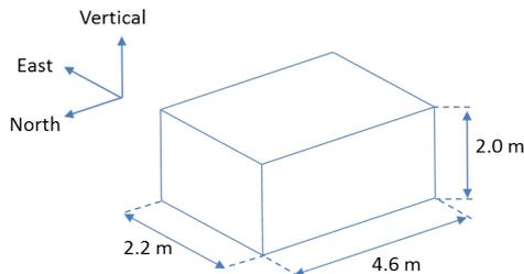
Figure 1: Diagram of the petawatt target chamber and its internal cavity dimensions without the metal clad shielding (25 mm). The laser-target interaction point is roughly situated to be the centre of the chamber.
