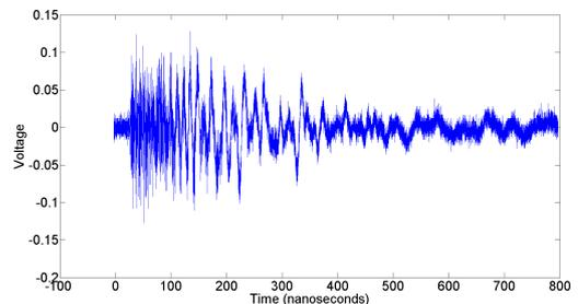
Figure 2: An example trace of EMP pick-up with a moebius loop [3] attached to an oscilloscope, displaying voltage as a function of time.
